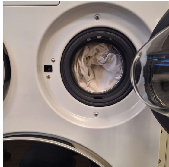
Fig. 3 – 1kg cotton load tested inside the small drum of the Multiwash
